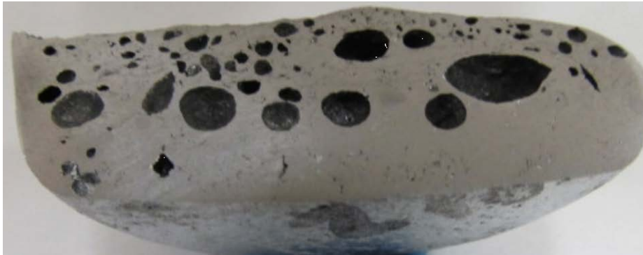
Untreated: RPT Density 2.18, AISCAN (0.365 ml/100g)
