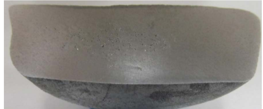
Degassed: RPT Density 2.66, AISCAN (0.128 ml/100g)
