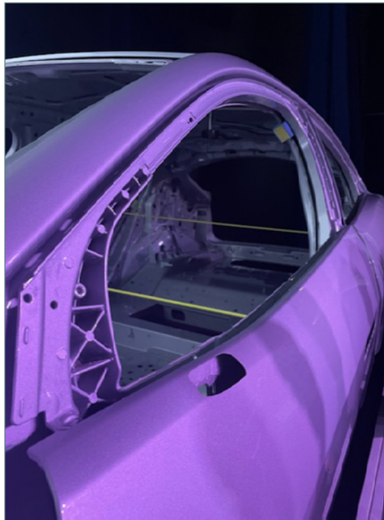
Figure 3. The door structure of the Jaguar I-Pace. (Photo: Mayflower Consulting.)
